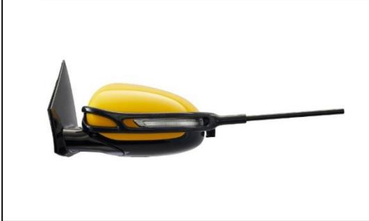
The image shows the yellow mirror housing with the black mirror holder attached. The holder is being pushed downwards from the top of the housing until it rests on the blinker mechanism.
