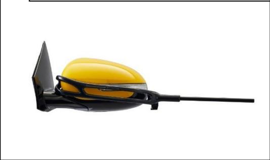
The image shows a side view of the yellow mirror housing. A black mirror holder is being inserted from the inside of the housing into a slot. The holder has a long, thin stem extending outwards.
