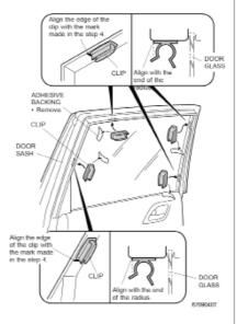
7. Repeat the procedure to install the clip on the right
