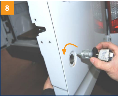
This retracts the safety catch. Turn the key counterclockwise and remove the lock housing.
