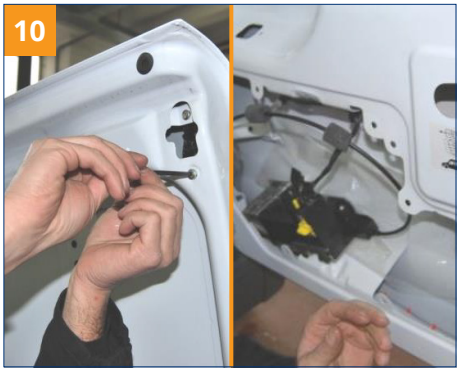
Unscrew the upper hook. Finally, remove the cable and the hook from the inside. Reinstall the lock in the rear door.
