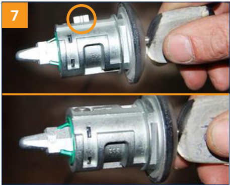
This retracts the safety catch. Turn the key counterclockwise and remove the lock housing.
