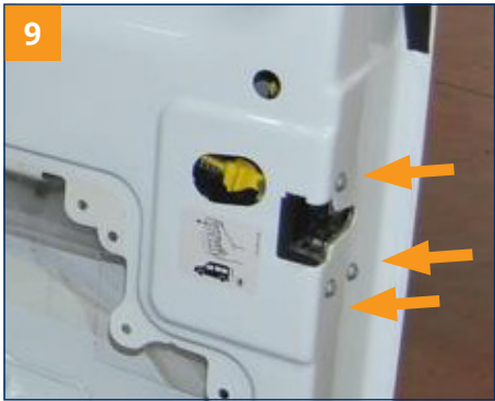
Loosen the lock fastening bolts.
