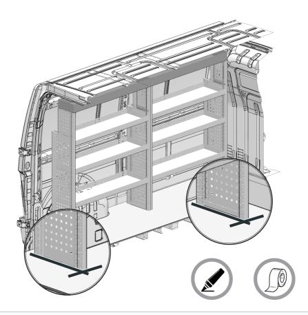
You can now move the cabinet aside. If there is interior paneling, it should also be removed in this step. We want to mount directly on the chassis without using the paneling.
