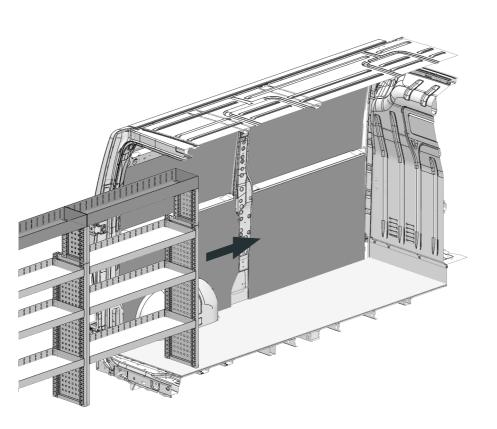
Now, make a mark on the floor for the position. Try to be reasonably accurate as this will reduce errors in the rest of the process. The most crucial aspect to mark is the distance from the wall, but also determine the depth along the length of the vehicle.
