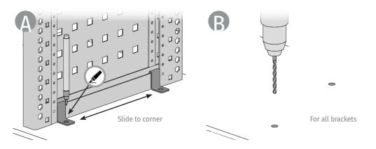
The paneling needs to have some holes to make sure the mounting brackets can be passed through.
