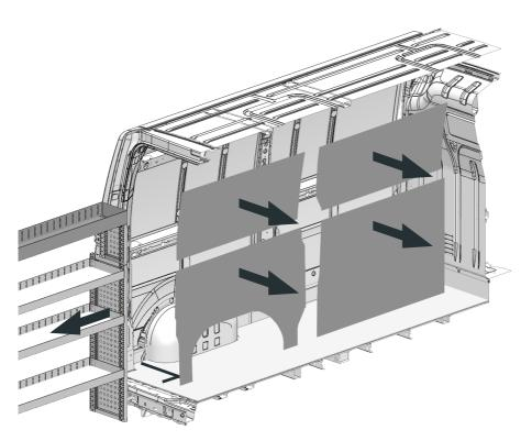
Now, place the cabinet back on the marking, and we will determine the position, as well as the bending, of the mounting brackets. This applies to all mounting brackets and the floor points. For wall mounting, it's advisable to find a strong chassis section with at least 2 mm thickness or with folded edges nearby, as these are the strongest points. We recommend finding a location for mounting on the floor, in the middle, and as high as possible.
