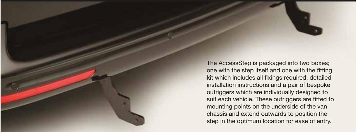
The AccessStep is packaged into two boxes; one with the step itself and one with the fitting kit which includes all fixings required, detailed installation instructions and a pair of bespoke outriggers which are individually designed to suit each vehicle. These outriggers are fitted to mounting points on the underside of the van chassis and extend outwards to position the step in the optimum location for ease of entry.
