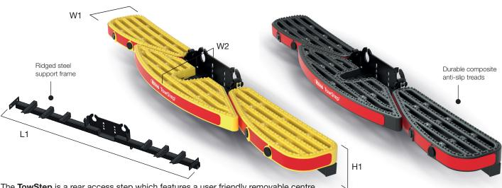
The TowStep is a rear access step which features a user friendly removable centre section, allowing a trailer to be attached effortlessly in a matter of seconds. This feature allows trailers to complete an impressive industry leading turning angle of 110 degrees. With the bolts provided, the TowStep can be fitted trouble-free to any flange type towbar.
