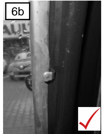
The holder is under the rubber put on the sheet metal
