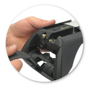
Attach clamp to each leg. NOTE; clamps may have labels showing their positions on the vehicle (For example; "Front Right").
