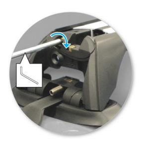
Tighten adjusting screw to 5 Nm (3.7 ft lb) hand tight.
