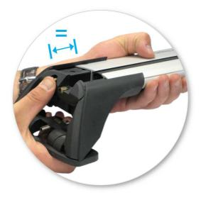
Press adjusting screw and pull crossbar legs out. Refer to the crossbar instructions for crossbar adjustment.
