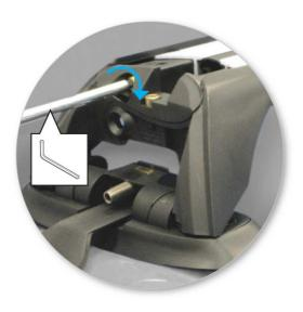
Tighten adjusting screw to 5 Nm (3.7 ft lb).
