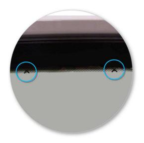
Locate vehicle fixed point for the rear bar as indicated on rear window.
